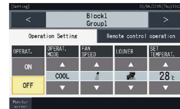
ON/OFF, "operation mode," "fan speed," "swing louver direction," "setting temperature," and "prohibition of remote control operation for individual items (run/stop, operation mode, fan speed, wind direction, setting temperature)"
